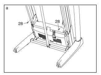
Lower the treadmill (see HOW TO LOWER THE TREADMILL FOR USE on page 23). Remove the five #8 x 3/4" Screws (10). Carefully raise the ends of the Left and Right Foot Rail Covers (49, 73) to remove two of the Screws. Then, carefully remove the Motor Hood (74).
