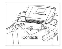
To measure your heart rate, **stand on the foot rails** and hold the metal contacts on the handrails for approximately ten seconds—**avoid moving your hands.** When your pulse is detected, first a heart symbol in the calorie display will appear; next, one or two dashes will appear; and then your heart rate will be shown. For the most accurate heart rate reading, continue to hold the contacts for about 15 seconds.
