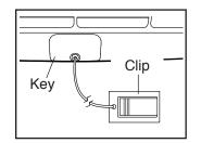
displays will light. **IMPORTANT: In an emergency**, the key can be pulled from the console, causing the walking belt to slow to a stop. Test the clip by carefully taking a few steps backward; if the key is not pulled from the console, adjust the position of the clip.
