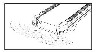
If the ultrasonic sensors detect an object, a message will appear in the display to alert you. If the object is in the zone closest to the treadmill, the walking belt will stop automatically.
