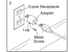
The lug or wire extending from the adapter must be connected with a metal screw to a permanent ground such as a properly grounded outlet box cover. **Some 2-pole receptacle outlet box covers are not** grounded. Before using an adapter, contact a qualified electrician to determine whether the outlet box cover is grounded. The temporary adapter should be used only until a properly grounded outlet can be installed by a qualified electrician.
